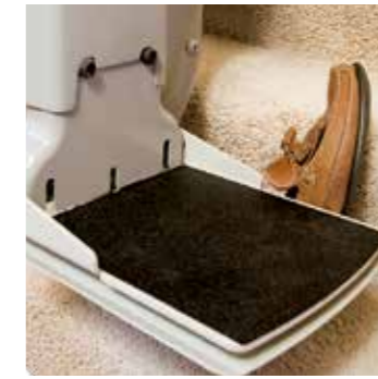
The foot plate and the carriage safety sensors stop the lift if an obstacle is in the way.
