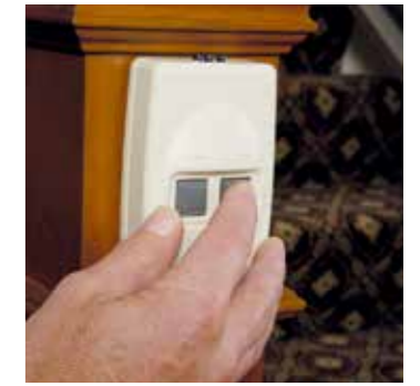
With the remote controls you can call or send the lift by pressing a button.
