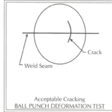
Figure 8a: Unacceptable Cracking. Figure 8b: Acceptable Cracking.
